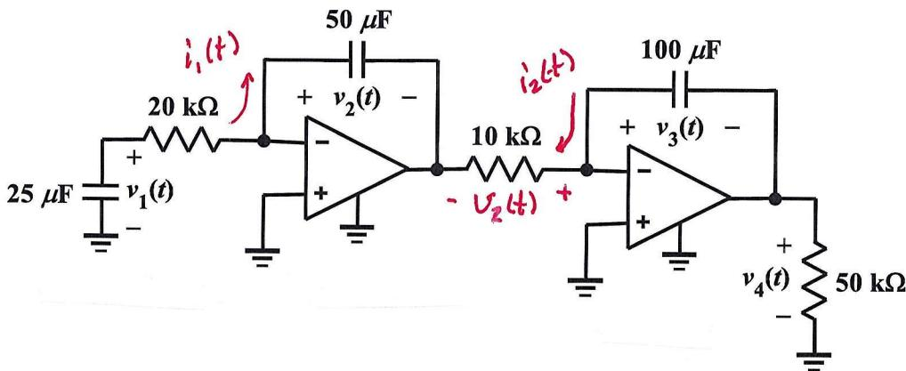
The operational amplifiers are ideal. If  $v_1(0) = 20 \text{ V}$ ,  $v_2(0) = -10 \text{ V}$  and  $v_3(0) = -5 \text{ V}$ , determine  $v_4(t)$  for  $t \geq 0$ .
